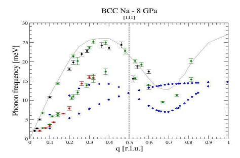
Figure 1: Phonon dispersion curves for Na at 0 GPa blue symbols (measured by neutron scattering by Woods, Brockhouse et al Phys. Rev. 128, 1112, 1962) and at 8 GPa black, red and green symbols measured during the experiment. Surprisingly, since 1962 the phonon dynamics of the alkali metals was not experimentally investigated even though recently sveral theoretical papers appeared: Rodriguez-Prieto, et al., Phys. Rev. B 74, 172104 (2006), Xie et al., *ibid*, 75, 064102 (2007).
