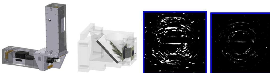
Figure 1. 3D Detector. From right to left: A sketch of the main part of the 3D detector comprising the two near-field screens. A close-up on the head showing the two screens and two mirrors. Experimental data from the two screens – evidently the pattern on the second screen – further from the source - is more reminiscent of a conventional powder diffraction pattern.
