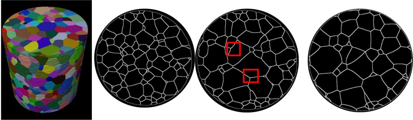
Figure 11. Coarsening of Ti. Left: experimental 3D grain structure before annealing. Colors only serve to visualize grains. Middle: one layer in the microstructure before annealing and after annealing. Right: same layer after annealing as simulated by an isotropic phase field simulation. One of the main differences between experiment and simulation is marked by the red boxes: in the experiment dihedral angles vary substantially, while they are fixed at 120 degrees in the simulations.
