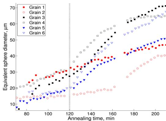
Figure 8. Growth rate of individual grains in aluminium during recrystallization. The vertical line marks when the temperature was increased.
