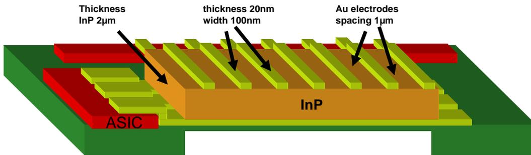
Figure 2. A sketch of the InP based nano-detector (not to scale)
