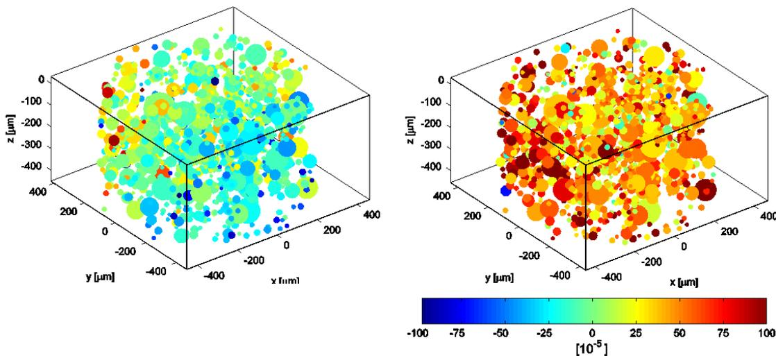
Figure 16. Centre-of-mass positions of 1118 grains in the mapped section of the cylindrical polycrystalline Cu sample plastically deformed under tensile load (along z) colour coded according to: Left) residual axial strain in undeformed sample, and Right) absolute axial strain at maximum load. The diameters of the spheres represent the relative grain sizes.
