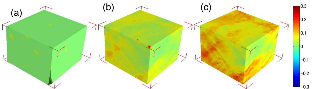
Figure 13. Plastic deformation of Al with Pb particles. Shown is the central part of the tensile specimen. Above: 3DXRD map of the undeformed sample. Colors denote orientations as defined by the stereographic triangle. Below: plastic strain maps from the same volume at a) 0%, b) 5% and c) 10% tensile loading. The colors symbolise the axial strain as shown to the right (red is tension). The resolution of the plastic strain maps is approx 20  $\mu\text{m}$ .
