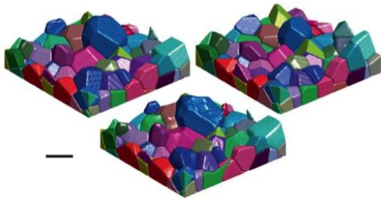
Figure 5.1. Top-left: 3D Laguerre tessellation based on the centers of mass and volumes from the 3D grain structure. Bottom: Segmented 3D grain structure. Top-right: 3D Voronoi tessellation based on the CMS from the 3D grain structure. Scale bar corresponds to 50  $\mu\text{m}$ .
