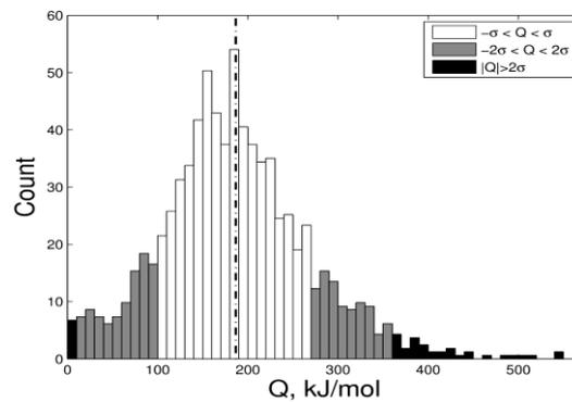
Figure 9. The distribution of grain-averaged activation energies of individual grains in aluminium during recrystallization. The vertical line marks the average, which is found to be consistent with values reported for bulk recrystallization.
