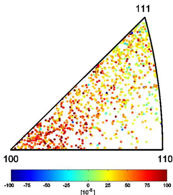
Figure 17. Stereographic triangle showing the orientation distribution of the 871 mapped bulk grains, colour coded according to their axial strain responses.
