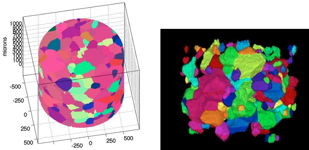
Figure 10. 3D grain reconstruction of grain growth experiment with C. Krill. Right: The microstructure after the last annealing is shown. Left: Bulk grains.
