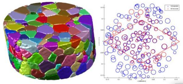
Figure 5.2. Left: 3D beta-tin grain structure from phase contrast tomography. Right: Subset of Boxscan and phase contrast tomography results plotted on top of each other. The size of the circles scale with grain radius. The red diamond is the scanned volume in the Boxscan experiment
