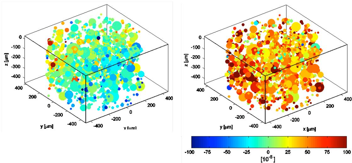
Figure 16. Centre-of-mass positions of 1118 grains in the mapped section of the cylindrical polycrystalline Cu sample plastically deformed under tensile load (along z) colour coded according to: Left) residual axial strain in undeformed sample, and Right) absolute axial strain at maximum load. The diameters of the spheres represent the relative grain sizes.
