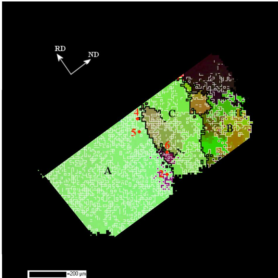
Figure 6. Nucleation in 30% cold rolled Al. Shown is an orientation map for one layer in the as deformed sample. The colours denote orientations. The white and black lines outline regions with misorientations above 2 deg and 15 deg, respectively. Grains A, B and C are identified. Supersposed as red dots are the center-of-mass positions of four new grains, which nucleated in or very close to this layer.
