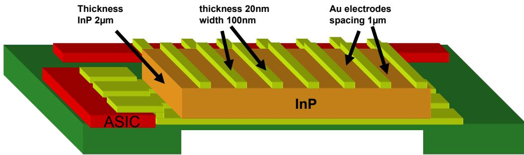
Figure 2. A sketch of the InP based nano-detector (not to scale)
