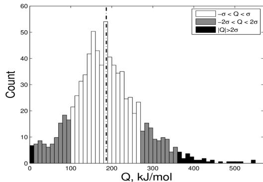
Figure 9. The distribution of grain-averaged activation energies of individual grains in aluminum during recrystallization. The vertical line marks the average, which is found to be consistent with values reported for bulk recrystallization.
