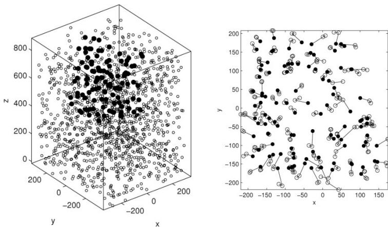
Figure 14. Left) Plot of the positions of the matched grains. Grains that could be tracked from 0% over 3 % to 9% are marked by filled symbols, while the symbols for grains that could only be followed to 3% are open. Right) The 107 grains tracked from 0% over 3% to 9% (filled) viewed along the tensile axis. The unit on the axes is  $\mu\text{m}$ .
