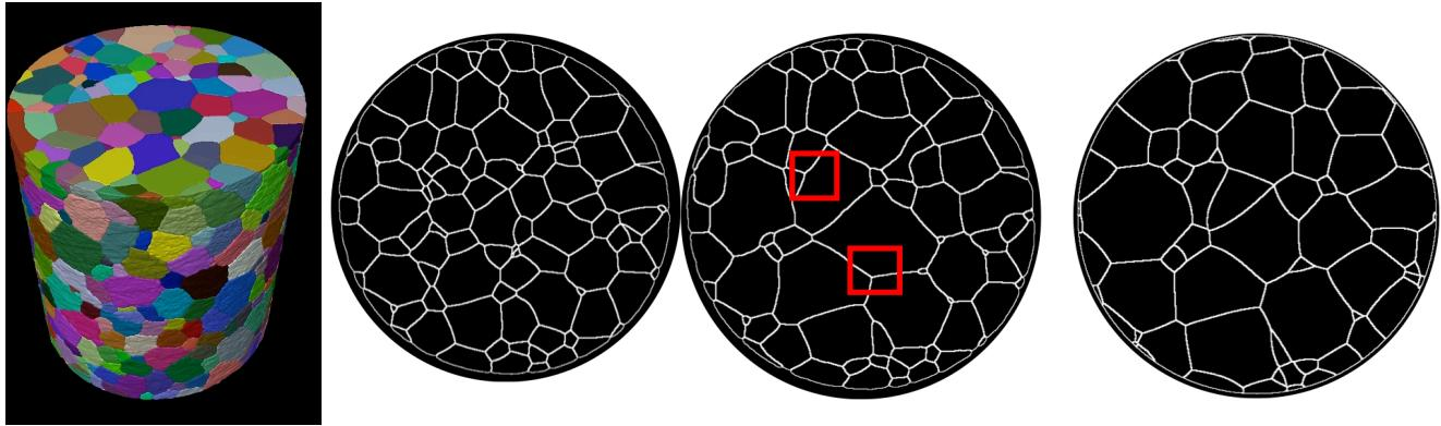
Figure 11. Coarsening of Ti. Left: experimental 3D grain structure before annealing. Colors only serve to visualize grains. Middle: one layer in the microstructure before annealing and after annealing. Right: same layer after annealing as simulated by an isotropic phase field simulation. One of the main differences between experiment and simulation is marked by the red boxes: in the experiment dihedral angles vary substantially, while they are fixed at 120 degrees in the simulations.
