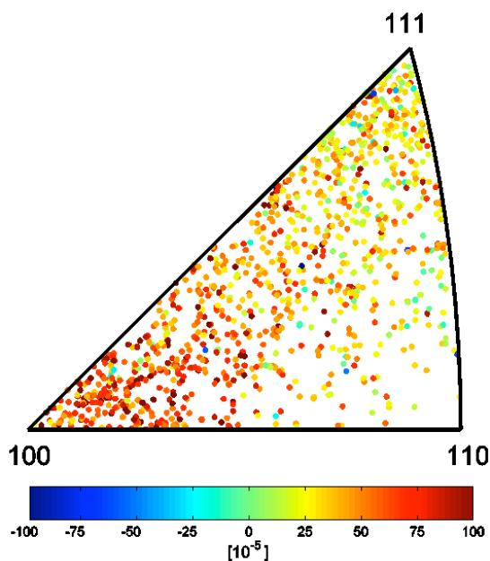
Figure 17. Stereographic triangle showing the orientation distribution of the 871 mapped bulk grains, colour coded according to their axial strain responses.
