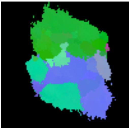
Figure 12. One layer of 10% tensile deformed sample reconstructed by GrainSweeper. Clear grain breakup is seen.
