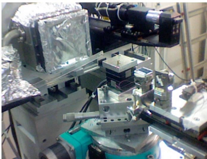
In order to overcome the stability problems in 2011 focus was on building a socalled **interim nanoscope**. This new station – placed at the end of EH3 – is essentially a hard x-ray optics platform. The platform has the required stability and enables a mounting of three detectors simultaneously. As shown in the photo above, on top of the platform in an ad hoc fashion
