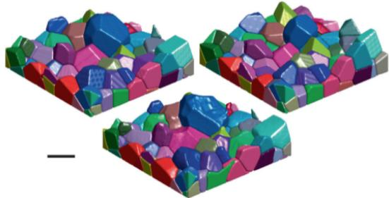
*Figure 5.1. Top-left: 3D Laguerre tessellation based on the centers of mass and volumes from the 3D grain structure. Bottom: Segmented 3D grain structure. Top-right: 3D Voronoi tessellation based on the CMS from the 3D grain structure. Scale bar corresponds to 50  $\mu$ m.*
