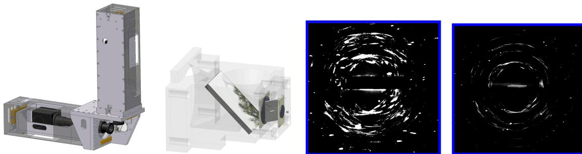
Figure 1. 3D Detector. From right to left: A sketch of the main part of the 3D detector comprising the two near-field screens. A close-up on the head showing the two screens and two mirrors. Experimental data from the two screens – evidently the pattern on the second screen – further from the source - is more reminiscent of a conventional powder diffraction pattern.
