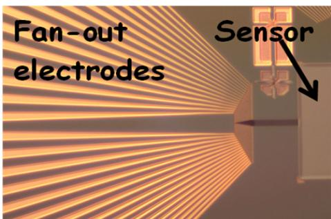
Figure 3. An SEM image of parts of the nano-detector made in the proof-of-concept study. The sensor itself is made by e-beam technology, the fan-out electrodes by UV-beam lithography. The figure is courtesy of the group of K. Yvind at DTU Photonics, Denmark, who is in charge of the clean-room work.
