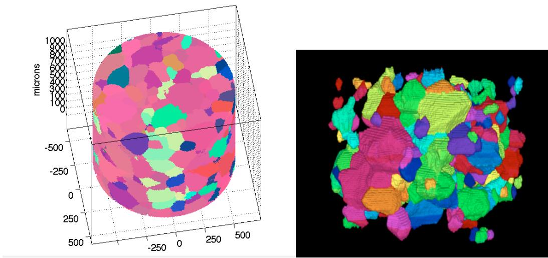
Figure 10. 3D grain reconstruction of grain growth experiment with C. Krill. Right: The microstructure after the last annealing is shown. Left: Bulk grains.
