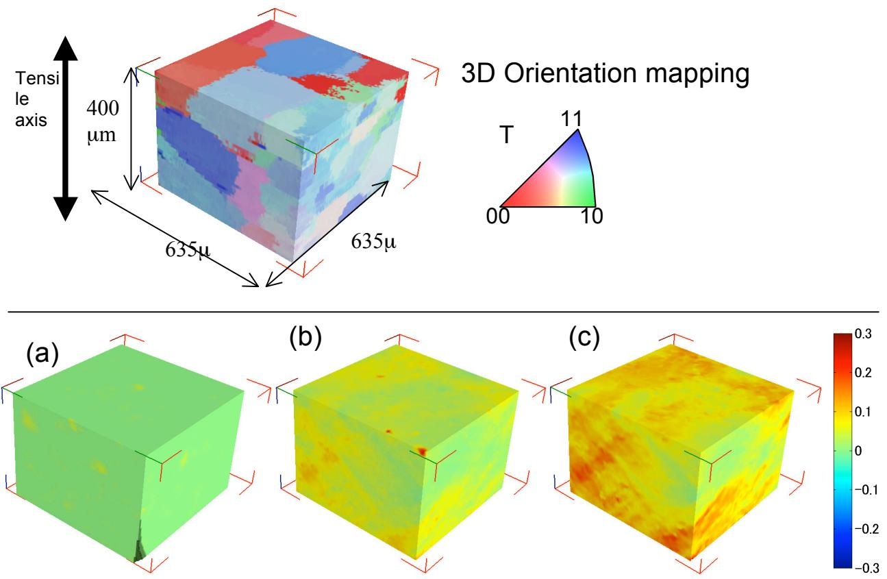
Figure 13. Plastic deformation of Al with Pb particles. Shown is the central part of the tensile specimen. Above: 3DXRD map of the undeformed sample. Colors denote orientations as defined by the stereographic triangle. Below: plastic strain maps from the same volume at a) 0%, b) 5% and c) 10% tensile loading. The colors symbolise the axial strain as shown to the right (red is tension). The resolution of the plastic strain maps is approx 20  $\mu\text{m}$ .
