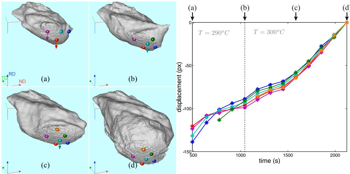
Figure 7. (a)-(d) Snapshots of the reconstructed 3D grain shape at different time steps during its growth. The length of the legs of the tripod corresponds to a length of  $42\ \mu\text{m}$ . (e) Displacement of local boundary segments perpendicular to the facet plane as indicated by the coloured markers in (a)-(d).
