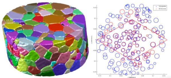
*Figure 5.2. Left: 3D beta-tinaium grain structure from phase contrast tomography. Right: Subset of Boxscan and phase contrast tomography results plotted on top of each other. The size of the circles scale with grain radius. The red diamond is the scanned volume in the Boxscan experiment*
