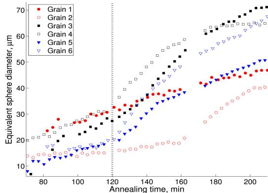
Figure 8. Growth rate of individual grains in aluminium during recrystallization. The vertical line marks when the temperature was increased.
