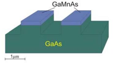
**Figure 1:** (GaMn)As/GaAs periodic wires ( $2\ \mu\text{m}$  period) on GaAs substrate
