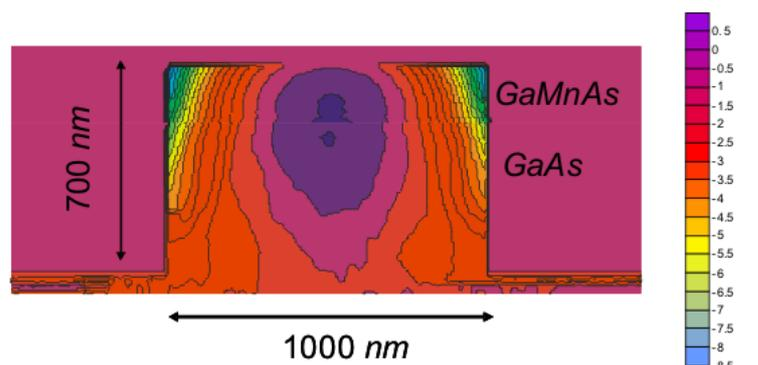
**Figure 3:** Retrieved vertical component of displacement field in (GaMn)As/GaAs single wire (in Å).
