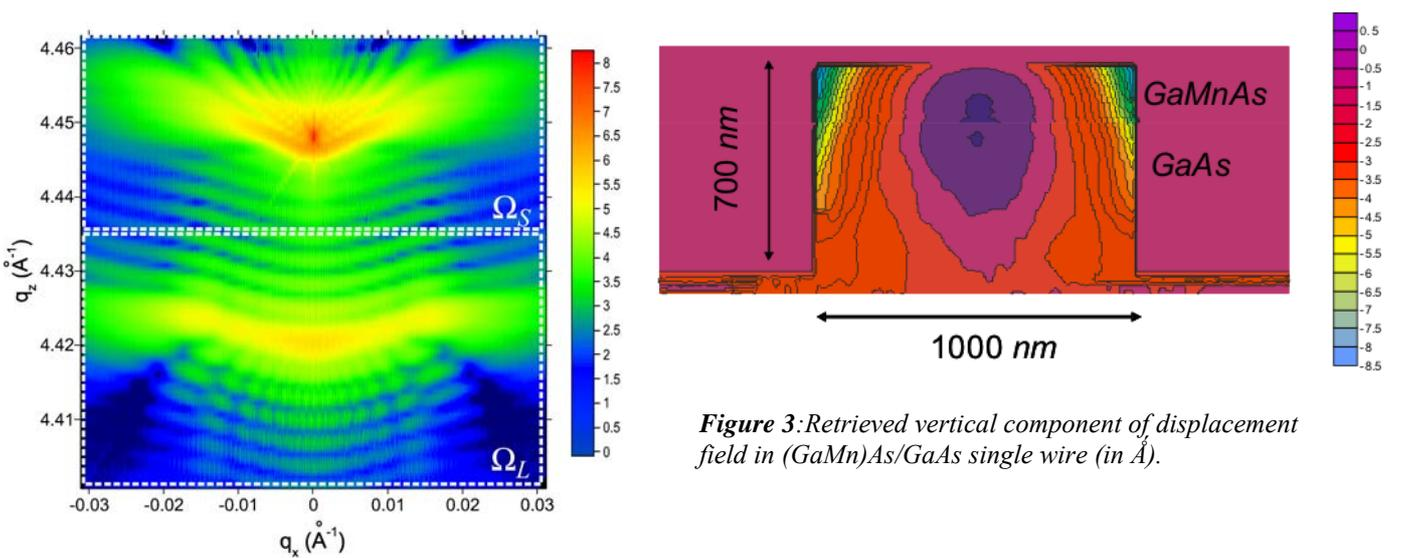
**Figure 2:** Reciprocal space map near 004 reflection of (GaMn)As (lower peak) / GaAs (upper peak) wires in the plane perpendicular to the etched wires direction.
