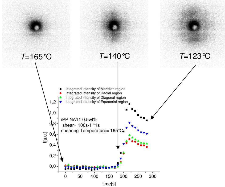
**Figure 1.** 2DSAXS images and integrated intensity of iPP-NA11 0.5wt% as a function of time after applying a shear of 100 ( $100\text{s}^{-1}$  for 1 s) at  $T=165^\circ\text{C}$ .
