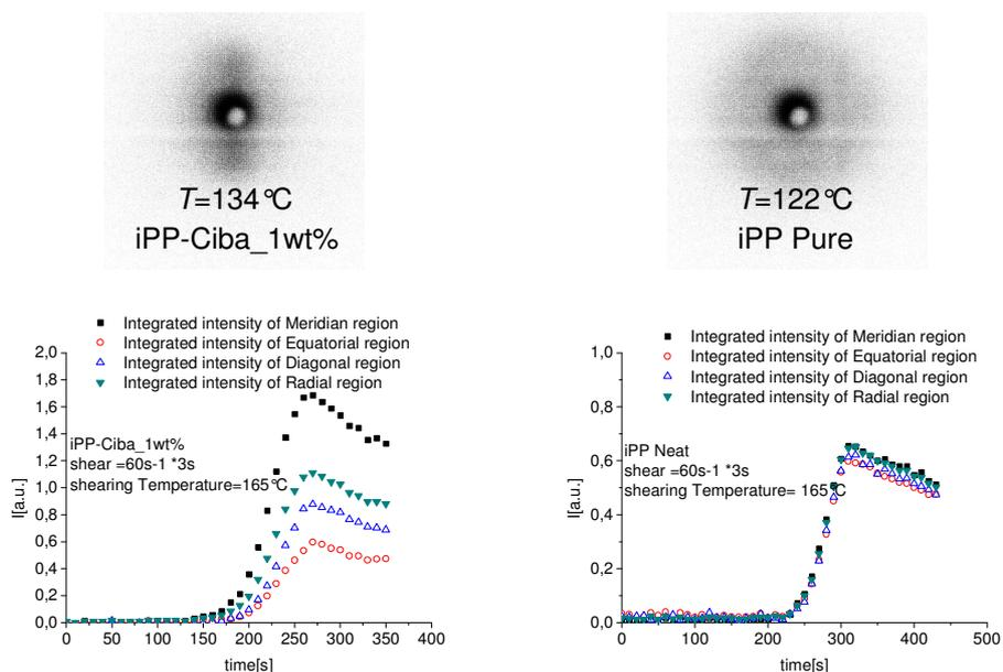
**Figure 3.** 2DSAXS images and integrated intensity of iPP-Ciba 1wt% and pure iPP as a function of time after applying a shear of 60 ( $60\text{s}^{-1}$  for 3 s) at  $T=165^\circ\text{C}$ .
