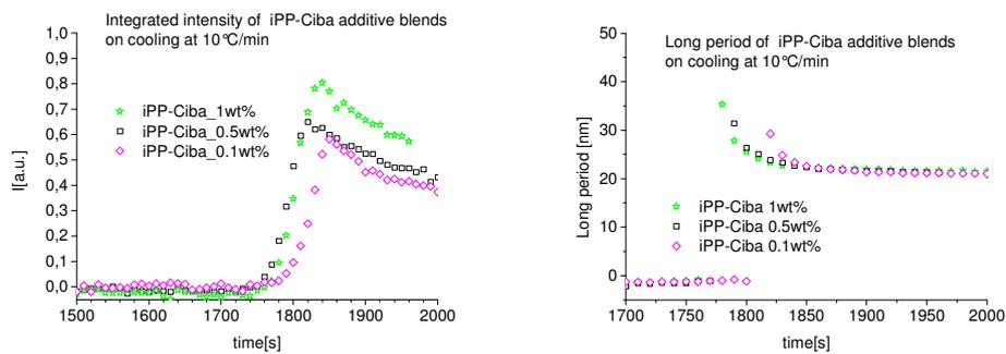
**Figure 2.** Integrated intensity (left) and long period (right) of iPP-Ciba blends as a function of time after cooling at  $10^\circ\text{C}/\text{min}$  during quiescent conditions.
