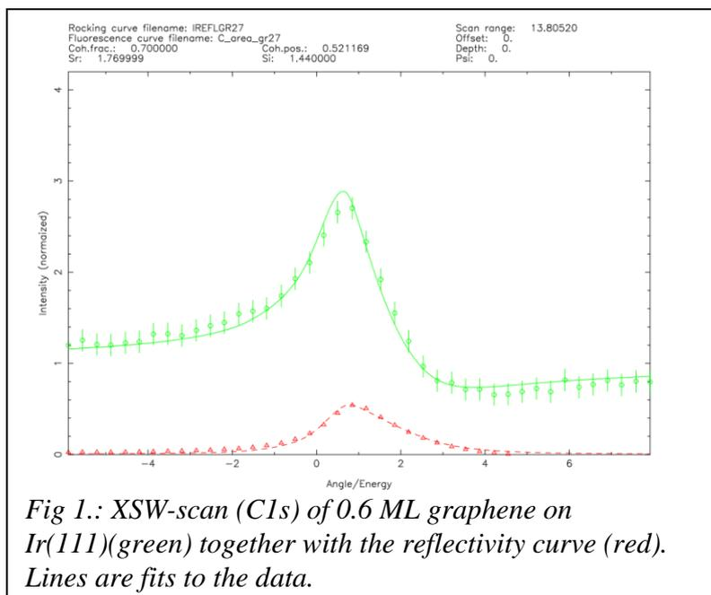
*Fig 1.: XSW-scan (C1s) of 0.6 ML graphene on Ir(111)(green) together with the reflectivity curve (red). Lines are fits to the data.*
