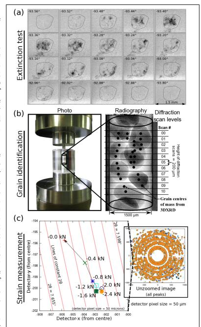
(a) Extinction test: radiographs after subtraction of the average of the first and last in sequence (to remove approximately direct beam image) at 0.04° steps from -93.56° to -92.80°. (b) Comparison of centres-of-mass from 3DXRD and grain positions from radiography (1.5 mm oedometer), (c) Movement of a selected Bragg peak, for a grain at the centre of the 10 mm oedometer sample, as a function of decreasing load.
