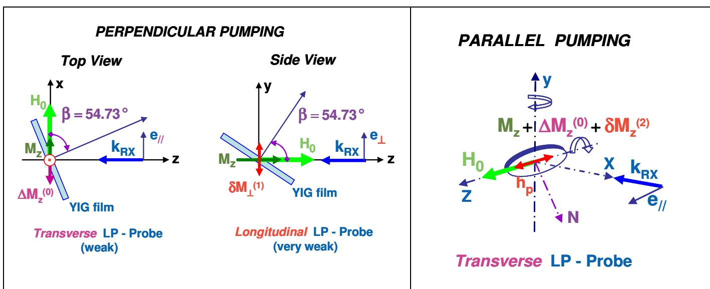
**Figure 1:** Alternative detection schemes for XDMR experiments under perpendicular pumping using Linearly Polarized (LP) X-rays. The normal to the film was arbitrarily rotated at the magic angle. The *transverse* geometry for the X-ray probe looks preferable (see text).
