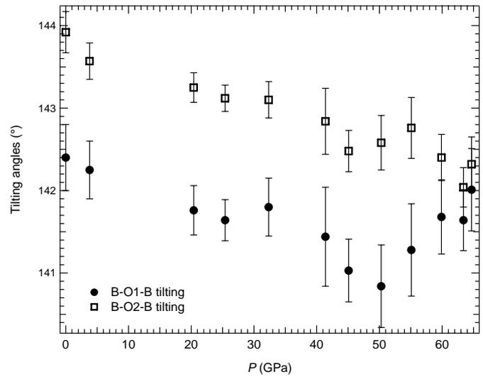
**Fig. 2:** Octahedral tilting angles of Fe-Al-bearing perovskite as a function of pressure
