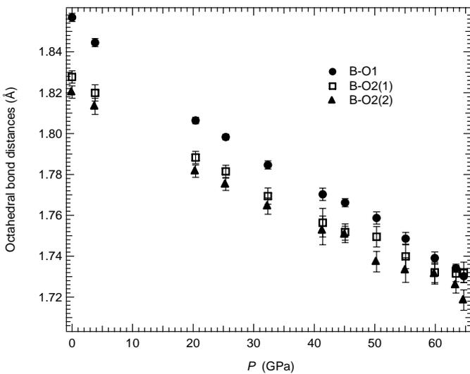
**Fig. 1:** Octahedral bond distances of Fe-Al-bearing perovskite as a function of pressure.
