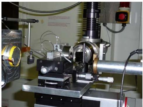
Fig. 1. The UniHead and DAC in “perpendicular” ( $90^\circ$  between the optical axes of the DAC and UniHead) geometry mounted on the goniometer at ID09a beam line.
