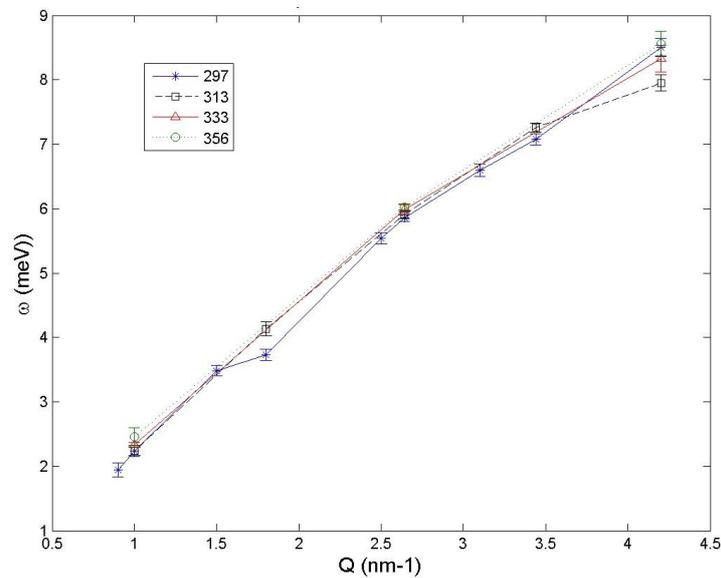
Figure 2: Dispersion curves obtained by fitting spectra at four temperatures
