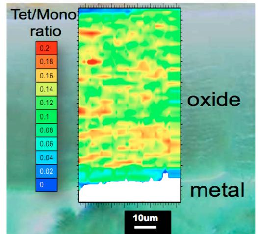
Figure 1: SEM micro-graph of oxide layers formed on ZIRLO (top) and Map of tetragonal/monoclinic peak ratio measured on oxide cross-section at ID13
