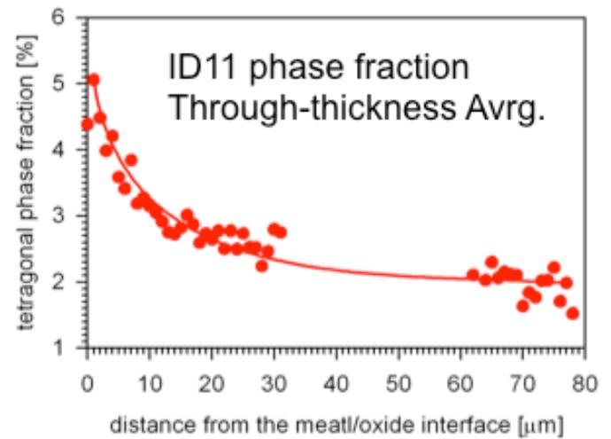
Figure 2: Tetragonal phase fraction as measured on ID11 – MA467 in transmission (through thickness average of 1mm sample)
