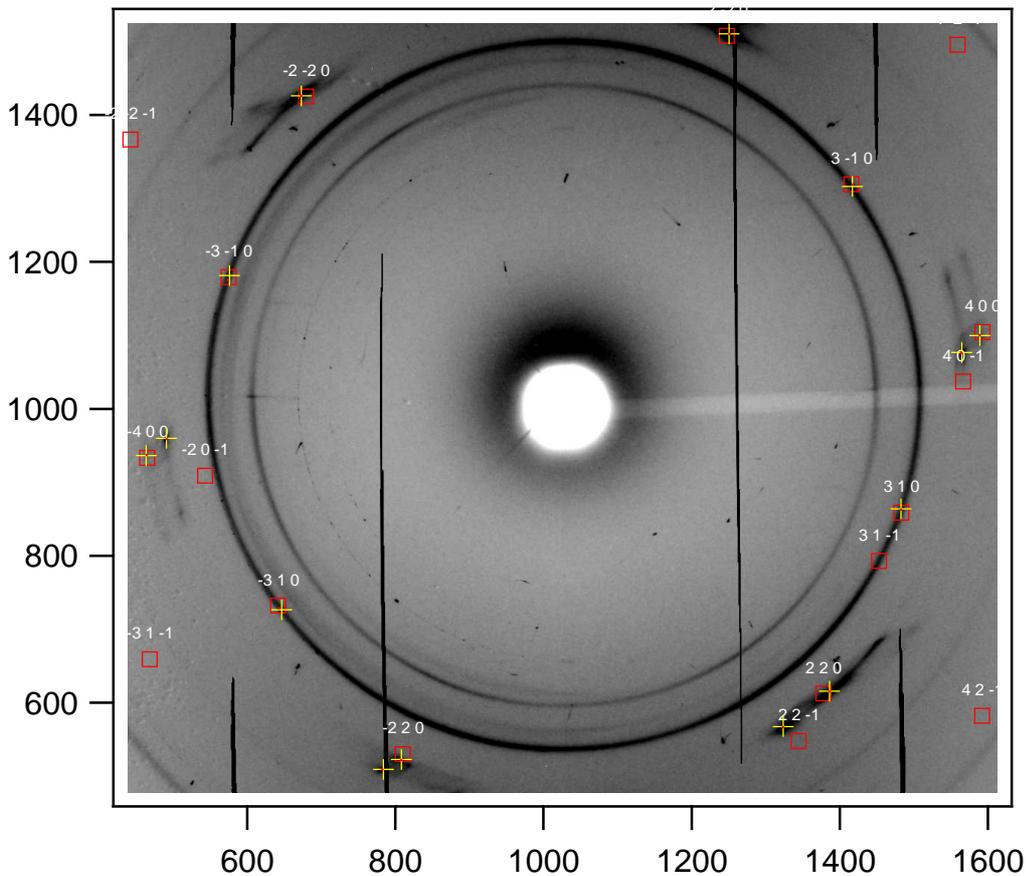
Figure 1: Panoramic X-ray diffraction pattern of oxygen at 187 GPa overlaid with the predicted (red square) and the observed (yellow cross) diffraction peaks.
