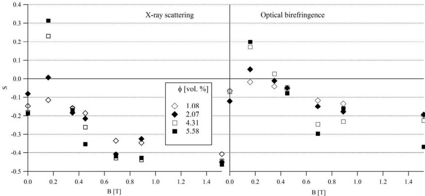
Figure 2: Order parameter  $S$  as a function of the magnetic field  $B$  applied during polymerization. (Left) Determined from the SAXS patterns. (Right) Determined from the optical birefringence of the samples,  $\Delta n$ . Different symbols correspond to different volume fractions  $\phi$  of goethite, indicated in the legend.
