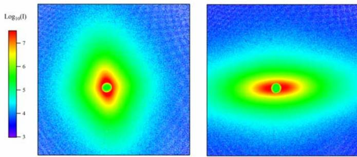
Figure 1: SAXS patterns for two samples polymerized under magnetic field. Left:  $\phi=5.58\%$  and  $B=0.2\text{ T}$  (alignment along the field,  $S>0$ ). Right:  $\phi=4.31\%$  and  $B=1.5\text{ T}$  (alignment perpendicular to the field,  $S<0$ ). No magnetic field was applied at the time of the measurement.
