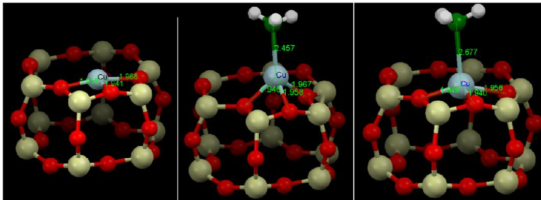
Figure 2. Illustrations of the local copper environment in  $d6r$  sub-unit of CHA. (a) Local structure after calcination with copper on the plane and slight distorted from the center of the  $d6r$  sub-unit of CHA; (b) interaction with  $\text{NH}_3$  at  $\sim 125^\circ\text{C}$  under SCR conditions resulting in a coordination geometry change; (c) under SCR conditions above  $250^\circ\text{C}$ .
