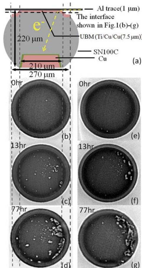
For comparison, Figure 3 shows the evolution of the interfaces of two unpowered solder bumps, which only suffered  $130^\circ\text{C}$  thermal aging. Compared to the image taken at 0hr, after 77hrs, there are also several small voids founded at the interface, which means the reaction between UBM and solder body can introduce
