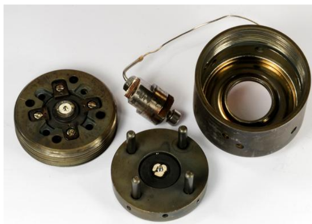
Figure 4 – The three principle components of an amagnetic DAC. From left to right; The base with attached solid diamond anvil, the top segment with perforated diamond, the helium gas membrane pressure drive.
