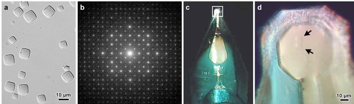
**Figure 1:** a) Optical micrograph of amylose V- $\alpha$ -naphthol single crystals; b) corresponding base-plane electron diffraction pattern; c) part of a Kapton cryoloop allowing to hold a thin vitreous film of aqueous crystal suspension; d) detail of the top of the Kapton loop indicated by the white square in c. the black arrows point to two single crystals embedded in vitreous ice.
