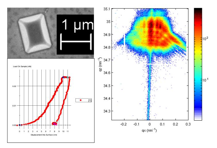
The diffraction pattern from this island does not differ a lot from the diffraction pattern from a regular pristine island, despite having undergone 8 nm of plastic deformation. It sets a lower boundary in the sensitivity of coherent x-ray diffraction in the sensitivity to crystal defects.
