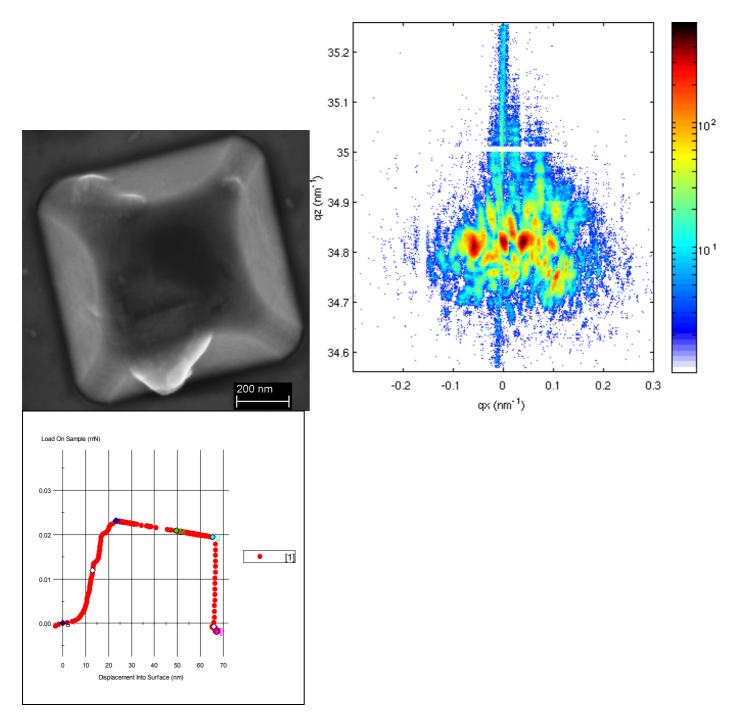
Here the crystal is so deeply indented that the imprint of the indenter is visible in the SEM image. The diffraction pattern is strongly affected, showing a lot of additional structures. Work is in progress to understand the nature of the defects that are responsible for these structures.
