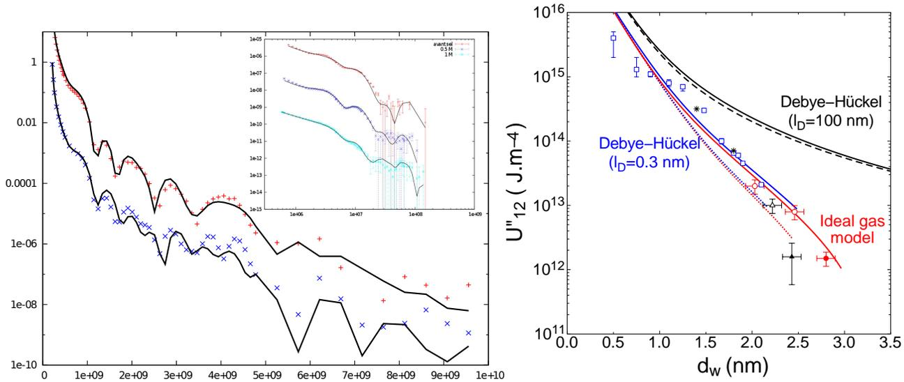
Fig. 1 : (left) Upper curve : specular reflectivity of a double bilayer in gel phase and best fit; lower curve : same sample
