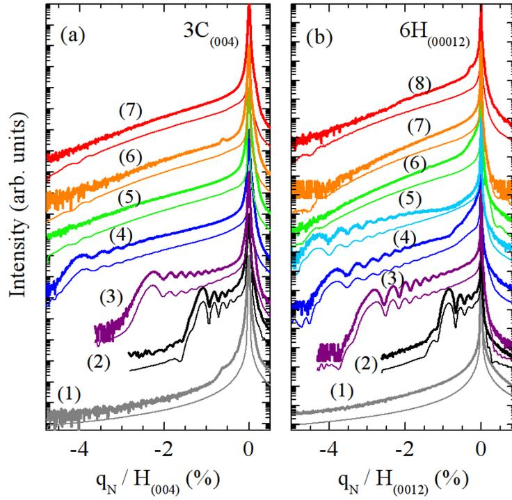
Figure 1: experimental (bold lines) and simulated (thin lines)  $\theta$ - $2\theta$  profiles recorded from 3C-SiC (a) and 6H-SiC (b) for increasing fluence.
