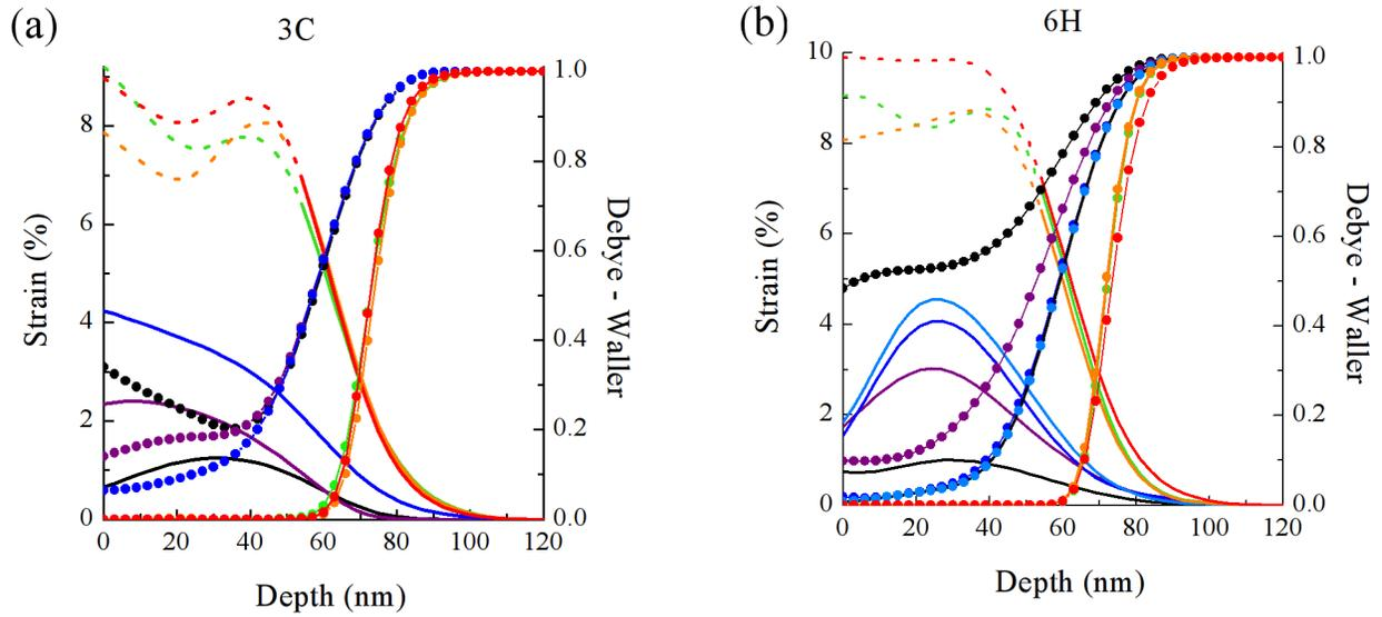
Figure 2 : strain and damage profiles obtained for 3C (a) and 6H (b) SiC (lines : strain, circles : Debye-Waller factor)
