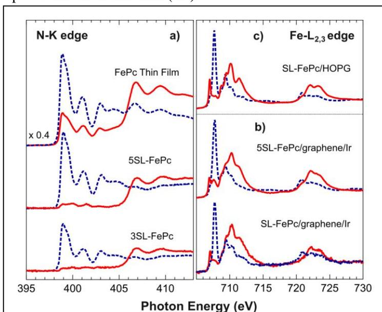
**Fig.1:** XLD data across the N-K edge (left, a) and the Fe- $L_{2,3}$  edges (right, b) and c), for FePc-graphene/Ir(111) at increasing FePc coverage (b). Data for the Fe- $L_{2,3}$  edge at FePc/HOPG is also reported (c), for comparison. Grazing incidence ( $70^\circ$ ) with linearly polarized radiation: total in-plane polarization (continuous red line); mostly out-of-plane polarization (blue dots).
