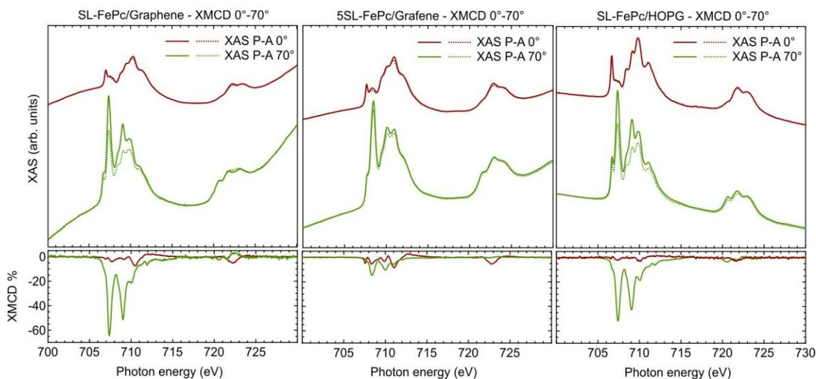
**Fig. 2:** (top panels) Fe- $L_{2,3}$  absorption data taken with circularly-polarized radiation parallel (red) or anti-parallel (blue-green) to the magnetic field, at  $0^\circ$  and  $70^\circ$  of incidence angle and  $H=5T$ ; (bottom panels) XMCD signals at  $0^\circ$  and  $70^\circ$  of incidence angle and  $H=5T$ . From left to right panels: 1 SL FePc on graphene, 5 SL FePc on graphene, 1 SL FePc on HOPG.
