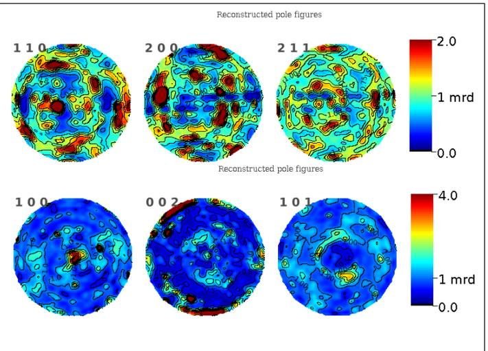
Figure 2: *(a) 110, 200, and 211 pole figures representing grain orientation statistics in  $\alpha$ -Fe in sample 2, before the first transition to  $\epsilon$ -Fe. (b) 100, 002, and 101 pole figures representing grain orientation statistics in  $\epsilon$ -Fe in sample 2, after the first transition from  $\alpha$ -Fe. Area projection, linear scale in multiples of a random distribution. Axial compression direction is at the center of the pole figure.*
