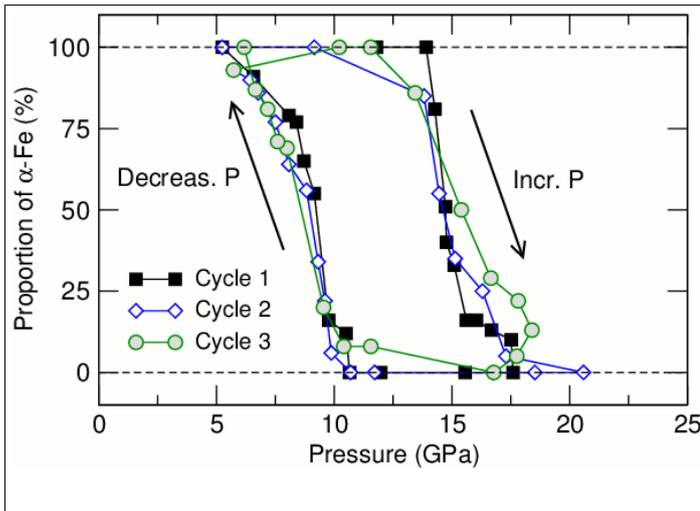
Figure 1: *proportion of  $\alpha$ -Fe as a function of pressure for the 3 subsequent cycles of pressure increase and decrease performed on sample 2, loaded in helium.*
