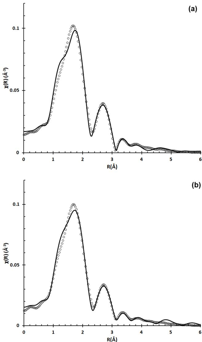
Figure 2: (a) Fourier transform of experimental (solid line) and simulated (circles) of the Ce K-edge EXAFS spectra on  $\text{Ca}_3\text{Sc}_2\text{Si}_3\text{O}_{12}:\text{Ce}^{3+}, \text{La}^{3+}$ . (b) Fourier transform of experimental (solid line) and simulated (circles) of the La K-edge EXAFS spectra on  $\text{Ca}_3\text{Sc}_2\text{Si}_3\text{O}_{12}:\text{Ce}^{3+}, \text{La}^{3+}$ .
