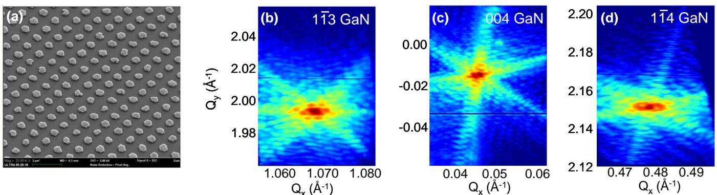
Fig. 1 (a) GaN nanowires (NWs) with a single dislocation (see black points at the center of the NWs in the scanning electron image) and/or inversion domain boundaries. (b)-(d) Two-dimensional reciprocal space images collected at different Bragg peaks for different GaN NWs.
