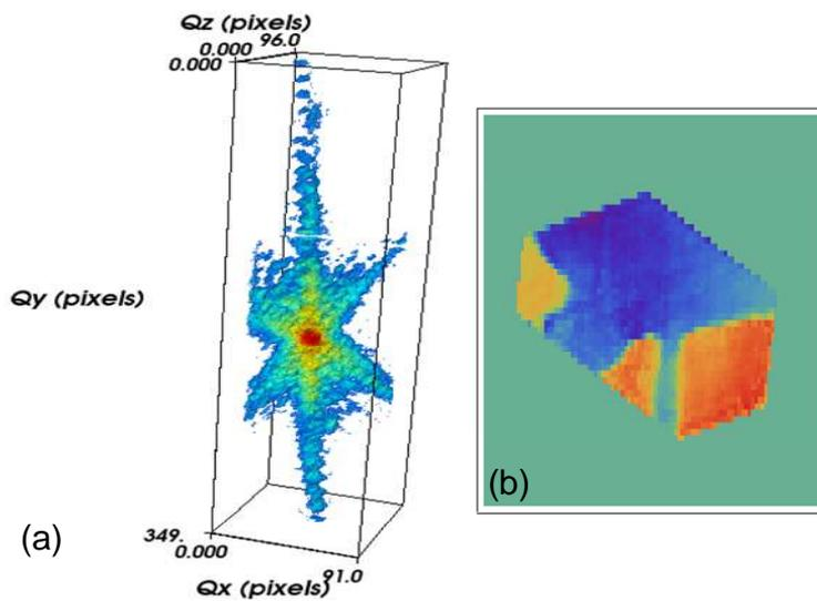
Fig.2 (a) Three-dimensional CXD pattern of the 004 reflection from a GaN nanowire. (b) Reconstructed phase, evidencing antiphase domains (the phase shift between the blue and the orange regions is  $\sim 2.8$  rad, the green region is outside the nanowire; the nanowire section is almost hexagonal, with main diameter 660 nm)
