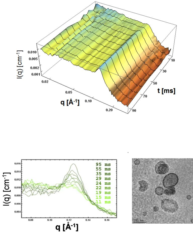
**Figure 1.** Millisecond range kinetic pathway of plasmid DNA (pDNA)/cationic lipid nanoparticle assembly revealed by time-resolved SAXS (4 ms exposure time), coupled to stopped-flow rapid mixing, and allowing for real-time monitoring of the complexes formation between pDNA and nanochannel-type fusogenic lipid carriers.
