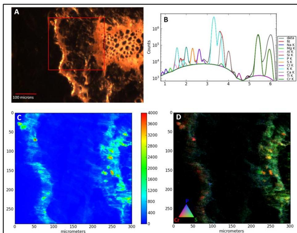
**Figure 1.** Cr distribution in the roots of seedlings germinated and grown for 15 days in 0.19 mM Cr(VI) and 1mM sulfate. A) Video microscope image of the root cross section (25 $\mu\text{m}$  thick). B) Fit of the map X-ray fluorescence sum spectrum. C) Cr K-edge X-ray fluorescence image acquired at 6.1KeV (2 $\mu\text{m}^2$  pixel), color bar scale in raw counts. D) Red Green Blue (RGB) image of Cr, S and P.
