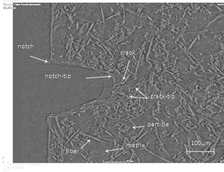
**Figure 2** Longitudinal section of the tomographic reconstruction at 136 MPa.
