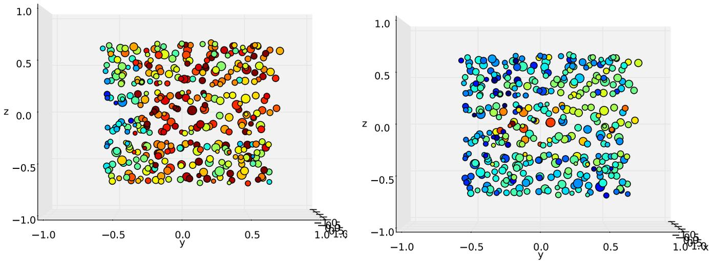
**Figure 1** Mg grains in the volume of interest at the maximum load with the notch to the left and the tip at  $z = -0.25$ . The left figure is colour coded according to the axial stress along the tensile  $z$ -axis, while the right is colour coded according to the stress along the  $y$ -axis – the growth direction of the crack.
