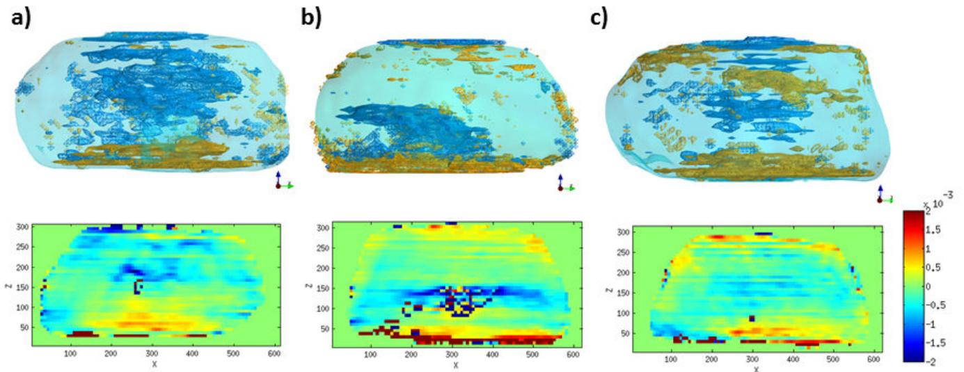
**Fig. 3:** Strain field calculated from the CBDi presented in Fig. 2 for a) the pristine Au crystal, b) after loading up to 2  $\mu\text{N}$ , and c) after measuring for 24h
