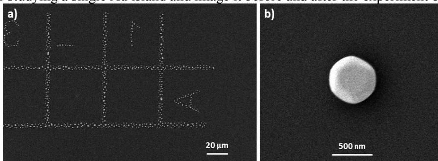
**Fig. 1:** SEM image of a) a regular array of Au crystals and b) a single Au crystal which was measured by *in situ* CBD.
