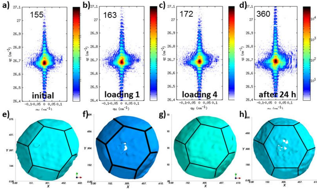
**Fig. 2:** Coherent Bragg different patterns of a) the pristine and the indented Au crystal loaded b) up to 250 nN, c) to 2  $\mu\text{N}$ , and d) after 24h of measurement. e) – h) Reconstructed images from the CBDi shown in a) – d)
