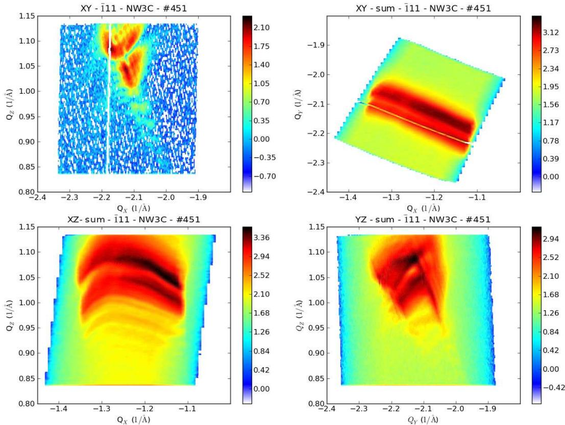
Fig. 2 Two-dimensional cuts of a three-dimensional rocking-curve around the 111 Ag Bragg reflection of a Ag-Au core-shell nanowire (see Fig. 1d).
