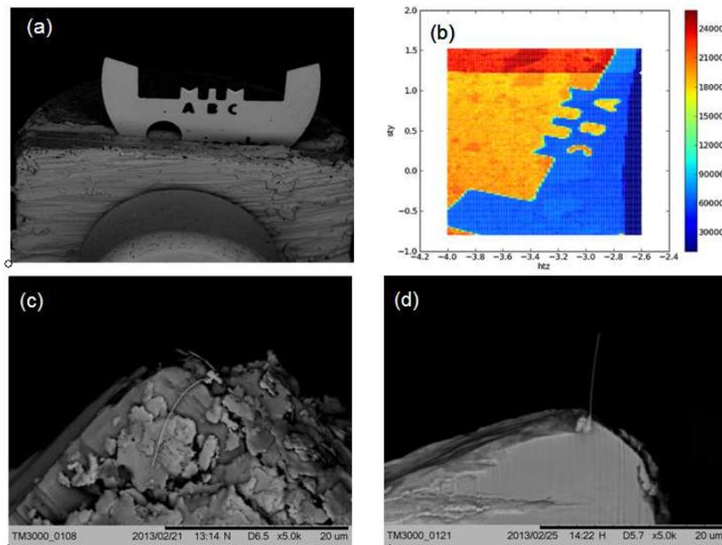
Fig. 1 (a) Scanning electron microscopy (SEM) image of the Mo TEM grid. (b) Image of the TEM grid obtained by scanning it in the direct beam. (c)-(d) SEM images of single nanowires on top of the TEM posts.
