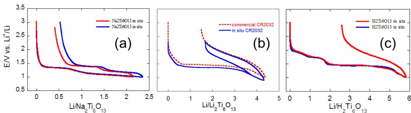
**Figure 1:** First discharge-charge cycle of Li cells using  $Na_2Ti_6O_{13}$  (a)  $Li_2Ti_6O_{13}$  (b) and  $H_2Ti_6O_{13}$  (c) as the positive electrode with *in situ* (blue) and commercial coin cells (red).
