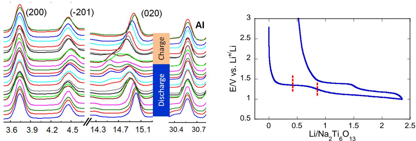
**Figure 2:** Typical *in situ* patterns collected during electrochemical Li insertion/de-insertion into  $\text{Na}_2\text{Ti}_6\text{O}_{13}$  together with the corresponding Li insertion curve.
