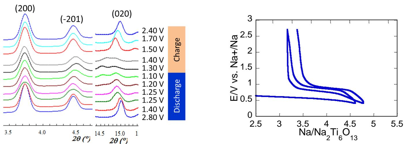
**Figure 3:** Typical *in situ* patterns collected during electrochemical Na insertion/de-insertion into  $\text{Na}_2\text{Ti}_6\text{O}_{13}$  together with the corresponding Na insertion curve.
