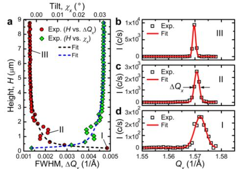
**Fig. 3:** (a) Full-width-at-half-maximum (FWHM) of the Ge(115) peak and tilt along the  $Q_x$  direction vs. crystal height. (b-d) Cross-sections through the Ge(115) peak along  $Q_x$  at 3 different crystal heights (e.g. I, II and III) depicted in (a).
