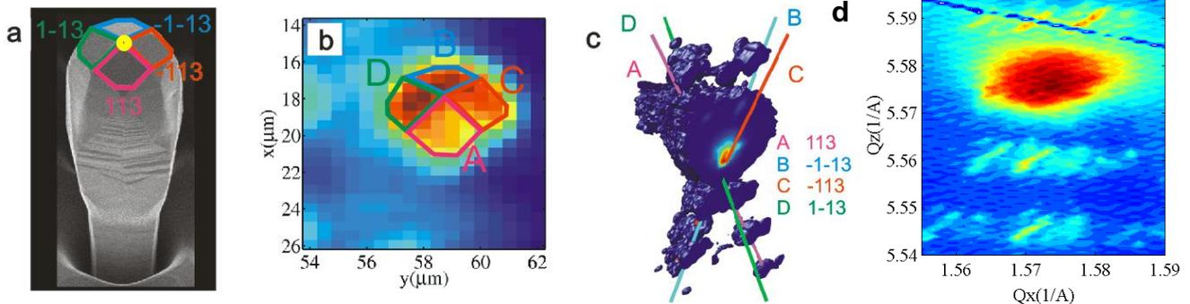
**Fig. 4:** (a) Perspective view SEM micrograph of a  $8 \mu\text{m}$  tall SiGe crystal with crystallographic facets, (b) the intensity maps scanned over the surface for all SL-1 peaks, the crystal facets shape is reconstructed, (c) 3D RSM around (115) reciprocal space point as iso-level surface plot recorded in the middle of the crystal. (d) example of the 2D RSM at selected point (yellow).
