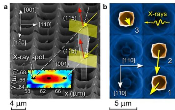
**Fig. 1:** (a) Scanning X-ray nanodiffraction of an isolated, 11- $\mu\text{m}$ -tall Ge crystal. The color map represents the scattered intensity collected around the Ge(115) peak when the incident beam was scanned along the crystal. (b) Top-view SEM micrograph of three Ge crystals showing schematically their tilt enhanced by a factor of 500.
