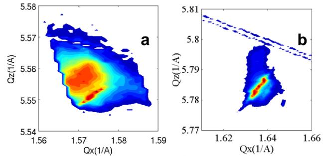
**Fig. 2:** Reciprocal space map around (115) for beam in the middle of the pillar: (a) signal from Ge - the narrow oblique peak is from crystal and the broad diffuse scattering originate from Ge in trenches, (b) signal from Si substrate.
