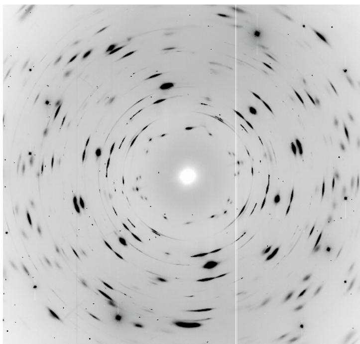
**Figure 1:** Diffraction pattern ( $\pm 33^\circ$  oscillation) of a quasi-single-crystal of Bi<sub>4</sub>Te<sub>3</sub> at 10 GPa.
