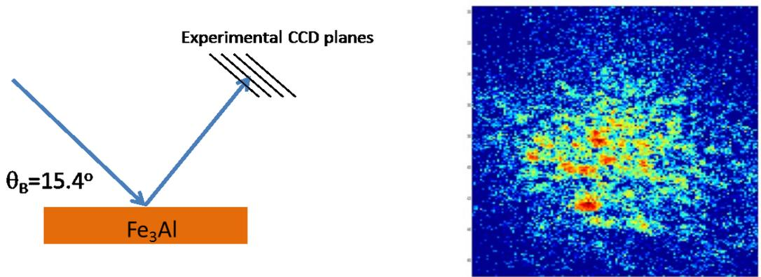
**Figure 1:** (left) sketch of the experimental setup. When the sample is rocked through the (001) reflection the experimental CCD planes sweep through the crystallite that is probed. (right) example of a speckle pattern from the (001) reflection.
