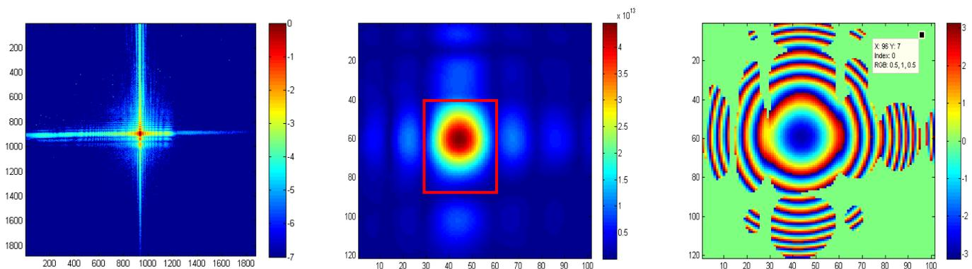
**Figure 2:** (left) measured intensity in the far field, (middle) back propagated beam amplitude at the sample position, (right) back propagated beam phase at the sample position. The beam size marked by the red square in the middle panel is about  $10 \times 12$  micron.
