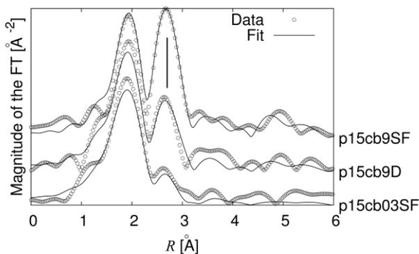
Figure 3: Fourier Transforms of the spectra presented in Fig. 2 with the related best fit curves. The transforms were carried out in the interval  $k=[2.6-9.5] \text{ \AA}^{-1}$  and the fit was carried out in R space on  $k^2$  weighted spectra in the interval  $R=[1.5-5.8] \text{ \AA}$ . The vertical line marks the position of the Ag-Ag bond that decreases for decreasing metal content.
