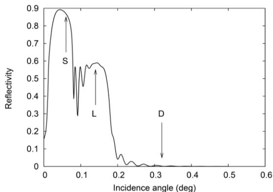
Figure 1: Reflectivity curve collected on sample p15cb3 at 25600 eV. The arrows mark the collection angles for RefEXAFS data: 0.06 deg for the Surface, 0.15 deg for the Layer and 0.32 deg for the Deep parts of the sample.
