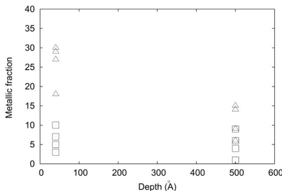
Figure 4: Metallic fraction values detected at the different sampling regions for the switched (triangles) and non-switched (squares) samples.
