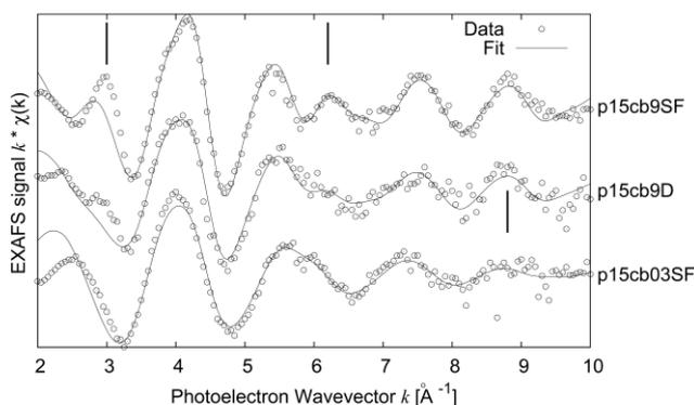
Figure 2: EXAFS spectra of 3 prototypical samples (switched p15cb09 in S and D collection mode and the non-switched p15cb03 in S mode) with the best fit curves. The vertical lines mark the features that grow for increasing Ag-metal content.
