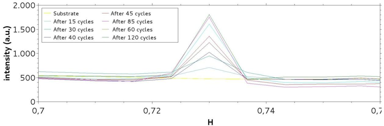
**Figure 1:** Evolution of the film observing the increasing of the intensity of the Bragg peak with the increasing of cycle number for the position  $H=0.73$ ,  $K= 0.73$ ,  $L=0.2$ .
