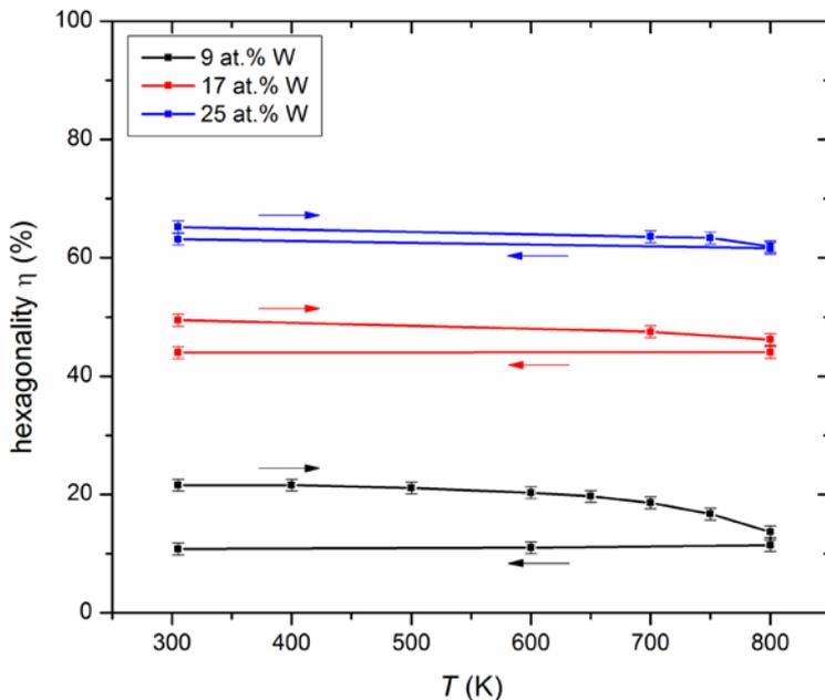
Figure 2: In-situ measurement results: Degree of hexagonality as a function of temperature for the three investigated Ni(W) films.
