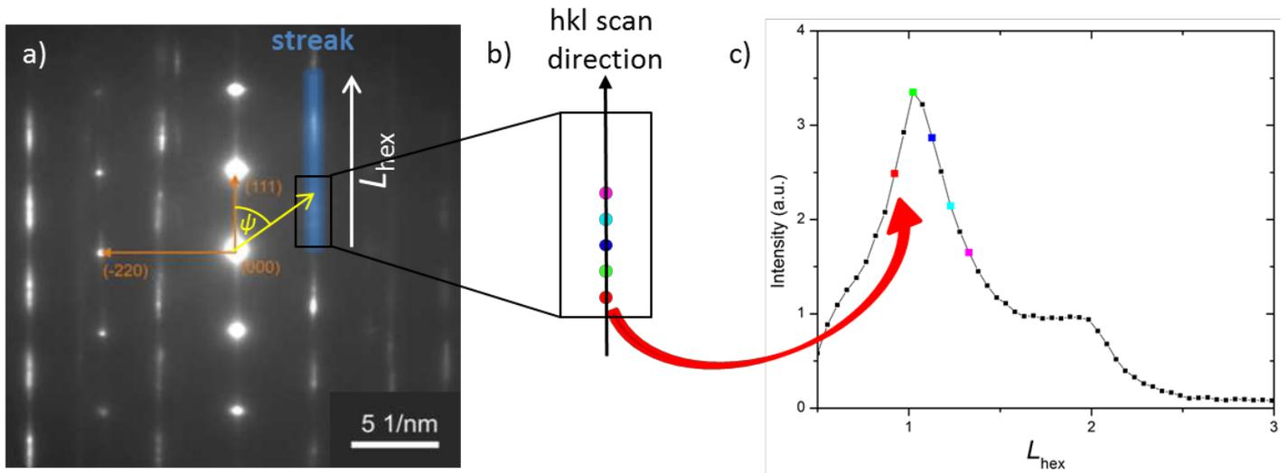
Figure 1: Illustration of the XRD measurement of the intensity distribution along the streak in the reciprocal space; a) electron diffraction pattern of a Ni(W) film showing the streaks in the reciprocal space; b) direction of the hkl scan, each color corresponds to a different  $2\theta$ - $\Psi$  pair; c) resulting intensity distribution on the  $L_{\text{hex}}$  scale.
