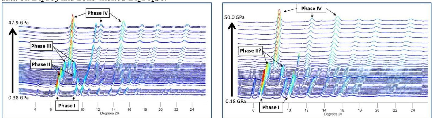
Figure 1. (Left)  $\text{Bi}_2\text{Te}_3$  upon compression to 47.9 GPa. (Right) Zone-melted  $\text{Bi}_2\text{Te}_2\text{Se}$  upon compression to 50.0 GPa.
