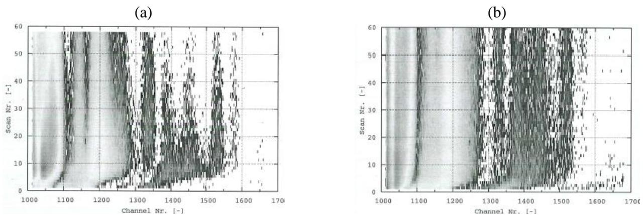
Fig. 2. Isothermal NFS scans (@ 300 °C) corresponding to the air (a) and wheel (b) side of the  $^{57}\text{Fe}_{81}\text{Mo}_9\text{Cu}_1\text{B}_9$  MG irradiated with the fluence of  $2 \times 10^{16} \text{ N}^+/\text{cm}^2$ .
