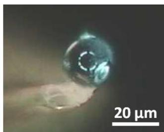
Figure 8. A mounted NIST SRM 2066 sphere.
