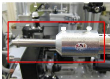
Figure 7. Confocal optic.
