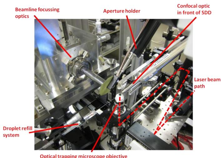
Figure 2. Detail of the OT setup on the beamline stages.
