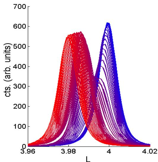
Fig. 1 – Temperature dependence of the (004)  $\alpha$ -U reflection from 20 K (blue line) to 200 K (red line) in steps of 5 K.
