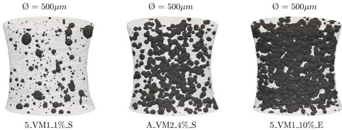
Figure 27 : 3D view of the samples prepared that were submitted to in situ tensile experiments.
