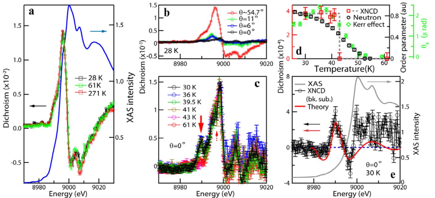
Fig. 1 X-ray absorption (XAS) and dichroic spectra measured at (a) selected temperatures and (b)  $\theta$ . (c) Dichroic spectra at low temperatures and  $\theta=0^\circ$ , showing the appearance of additional features. (d) Intensity of the dichroic feature marked by the big red arrow in c), compared with the square root of the spin ordering
