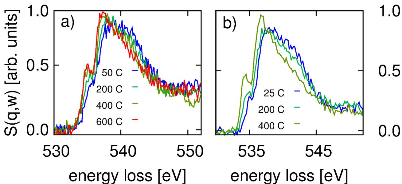
Figure 1: a) Results of the current experiment: O K-edge spectra of aqueous 34 m.% NaOH solutions for different temperatures and pressures. b) Results of a previous experiment: O K-edges from 14 m.% aqueous solutions of HCl.
