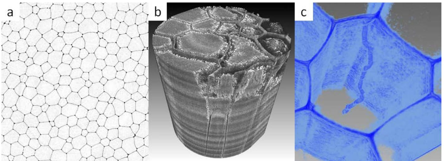
**Figure 1:** (a) – Reconstructed slide of a native sample, phase contrast; (b) – 3D spatial arrangement of partly etched calcite prisms surrounded by organic matrix, volume rendering; (c) – Segmented organic material of a native sample showing a canal connected to the interprismatic matrix, volume rendering
