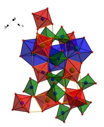
Figure 1: Typical view of a garnet-type structure with three cation sites: octahedral in red, tetrahedral in green and dodecahedral (twisted cube) in blue.
