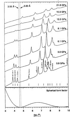
Figure 1. Pressure variation of the X-ray diffraction profiles of solid  $(C_{59}N)_2$  at ambient temperature from 0.8 to 21.8 GPa ( $\lambda$ = 0.5739 Å). The observed reflections (space group  $P6_3/mmc$ ) are labelled for the 0.8 GPa profile with the ticks below marking their positions. The bottom panel shows the calculated X-ray scattering form factor for quasi-spherical molecules of radius R= 3.55 Å.
