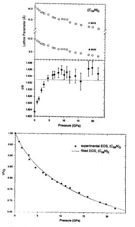
**Fig. 2** Pressure dependence of (a) the hexagonal lattice constants a and c and (b) the (c/a) ratio. The broken line marks the ideal value for a hcp structure.
