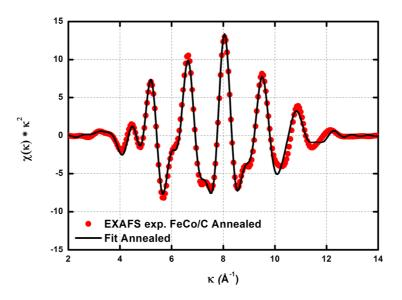
Figure 2 - EXAFS oscillations for FeCo 600V annealed at the Co K-edge (red spots) with best Fit (black line).
