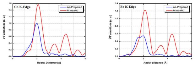
Figure 1 - Radial distribution of as-prepared (blue) and annealed (red) EXAFS signal at the Co K-edge (left) and the Fe K-edge (right).
