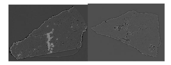
Figure 1. Phase tomographs of a carbonado from CAR (left) and of polycrystalline diamond from kimberlite.
