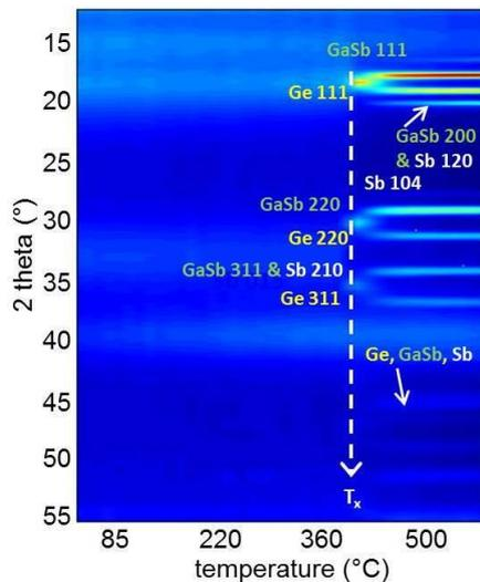
Figure 2: *in situ* XRD ( $\lambda=1.074$  Å) on medium Ge-doped GaSb ( $\text{SiO}_2$  capped).
