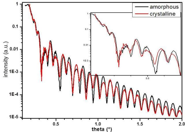
Figure 3: XRR ( $\lambda=1.074$  Å) before and after annealing of low Ge-doped GaSb layer ( $\text{SiO}_2$  capped). The inset is a zoom on the total reflection edge.
