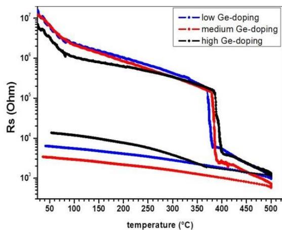
Figure 1: Sheet resistance for Ge doped Ga-Sb alloys as a function of temperature (ramp 2°C/min) and subsequent cooling to room temperature.
